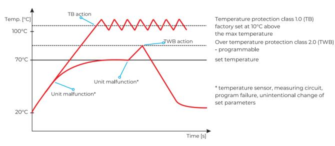
Over temperature protection class. 1.0 to DIN 12880 is a standard function for the ST/CHL/CL/IL/SL/SR/KK/CALDERA and SIMPLE equipment. It is factory set at approx. 10°C above the max temperature. Over temperature protection class 2.0 to DIN 12880 is a standard function for the CL/IL/SL/SR equipment in the Smart version.
