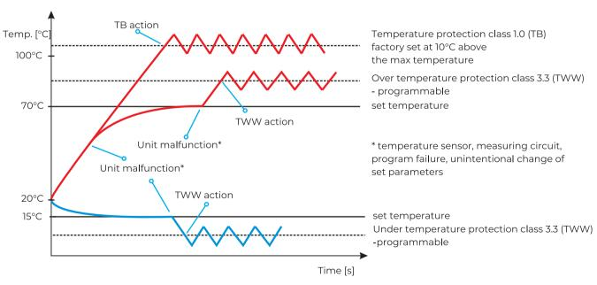
Over/under temperature protection class 3.3 to DIN 12880 is a standard function for the KK, ST and IL in the Smart PRO version. It is an additional option for ST and IL in the Smart version.
