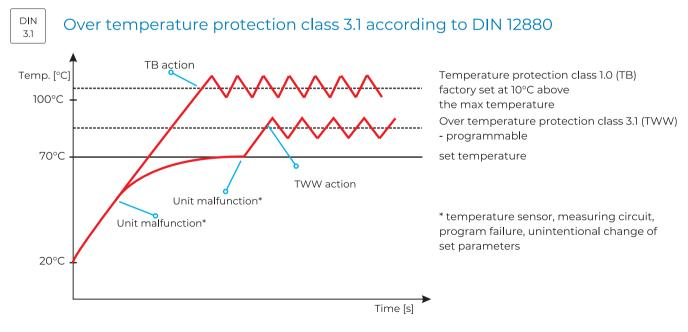
Over temperature protection class 3.1 to DIN 12880 is a standard function for the CL/SL and CALDERA equipment in the Smart PRO version, and optional for the CL/SL/SR ranges in the Smart version.
