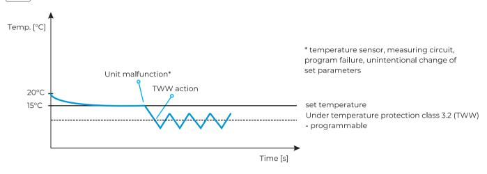
Under temperature protection class 3.2 to DIN 12880 is a standard function for CHL Smart PRO version and optional for CHL in Smart version.
